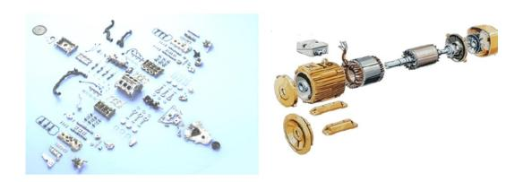
A combustion engine contains approximately 1400 different parts, whereas an electric motor consists in 210 parts. Electric mobility is, despite of the battery management, much simpler and demands much less labour. We are facing an enormous transition process.
